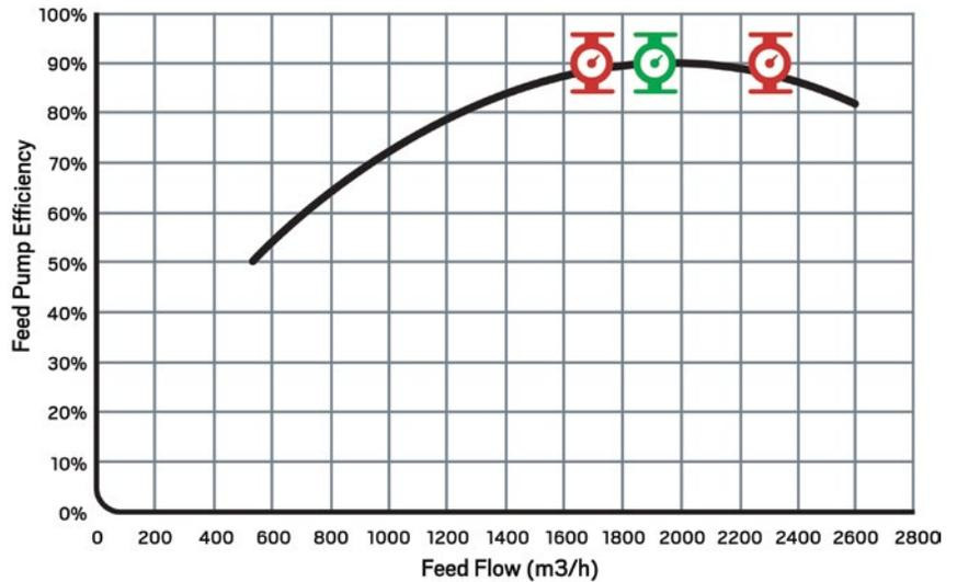
**With replaceable volutes, the AT Turbocharger can accommodate flexible flow rates, which can translate into millions of dollars saved in operating expenses**
