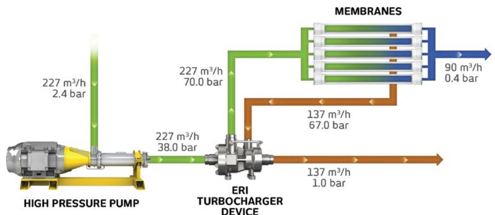
**This simplified process flow diagram shows how the Energy Recovery AT Turbocharger fits into the configuration of a typical desalination plant**
