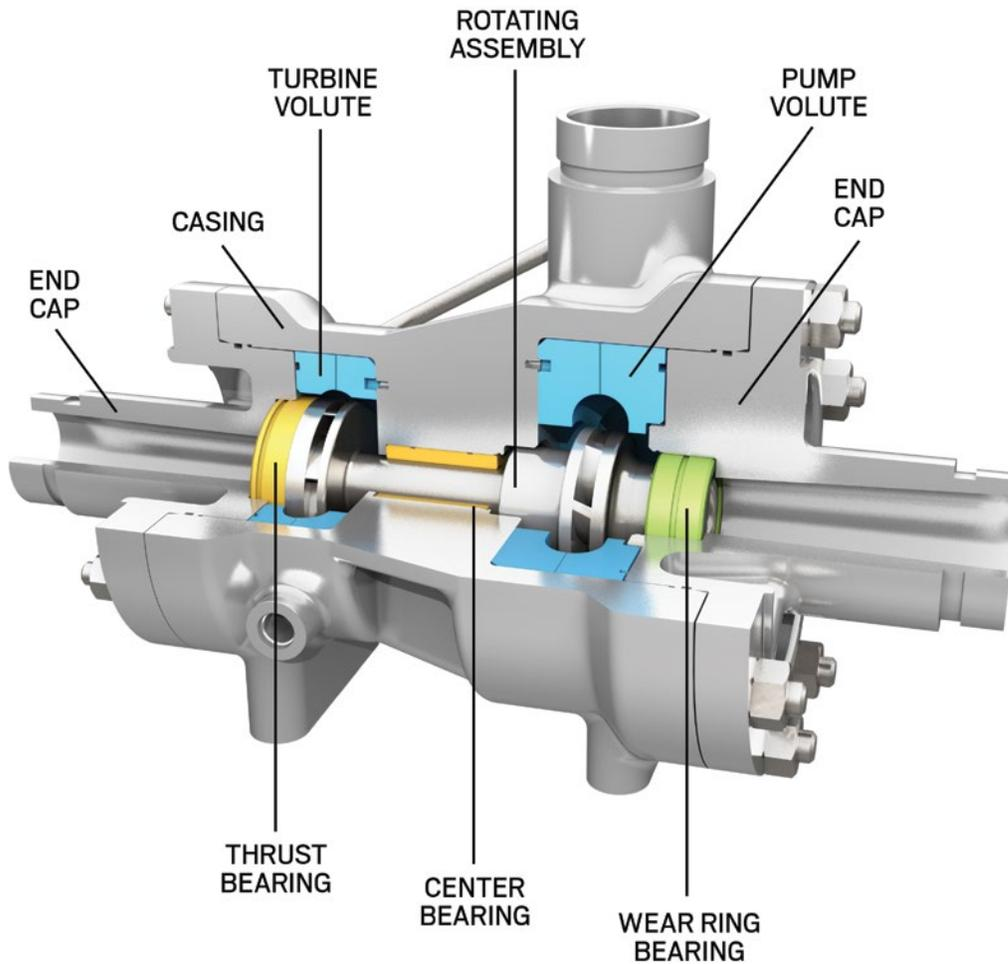
**A cutaway of the AT Turbocharger shows the solution's single rotating assembly and removable volutes**
