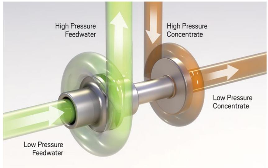
**Pressure energy is recovered by the AT Turbocharger through a fluid-to-fluid transfer of energy, from high pressure brine to the low pressure feedwater**
