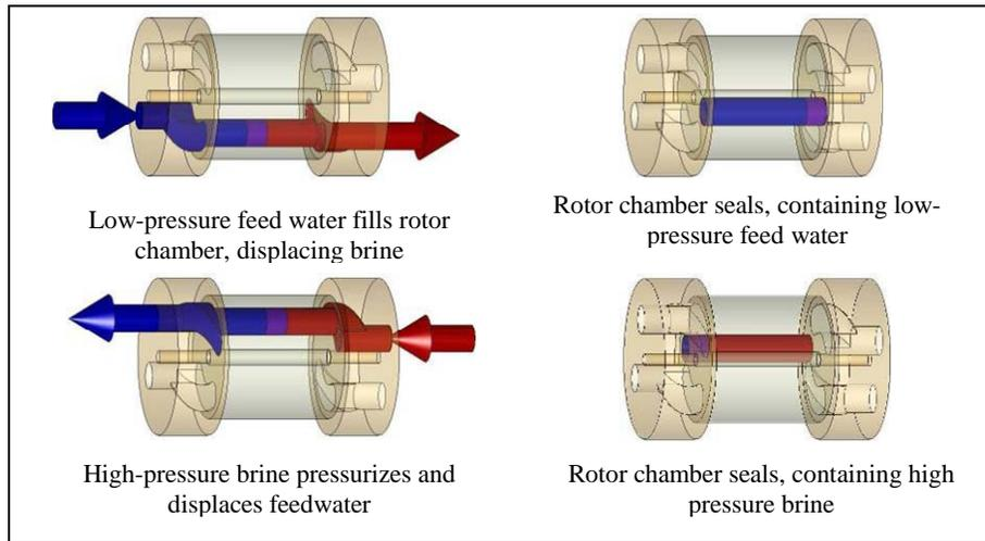
Figure 6 – Schematic Flow path through a PX unit
