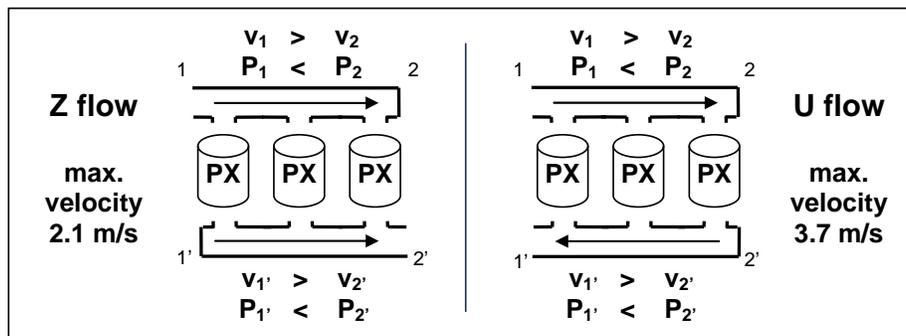
Figure 7 – Manifold flow Schemes
