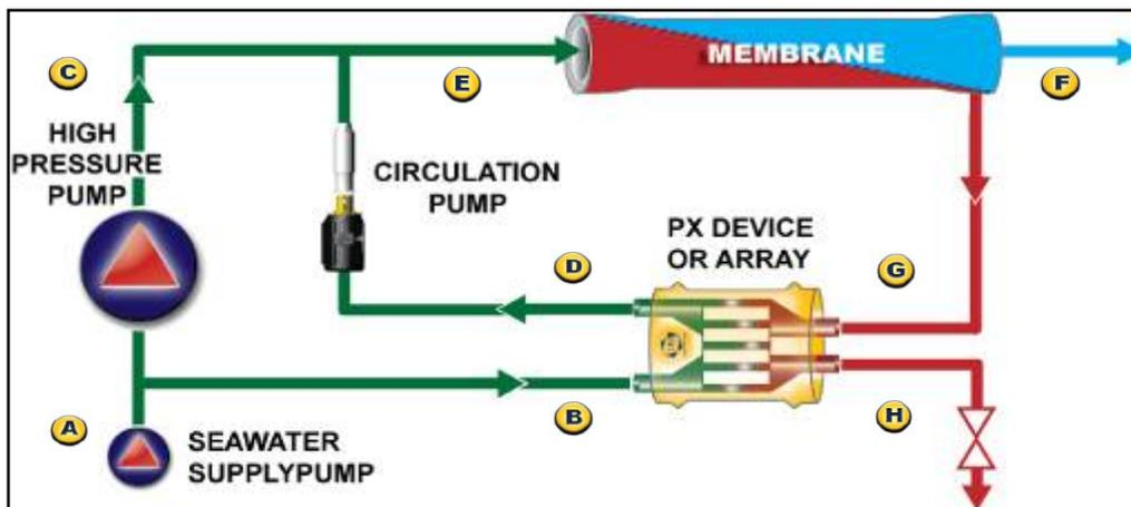
Figure 5 – Schematic Diagram of the SWRO Process
