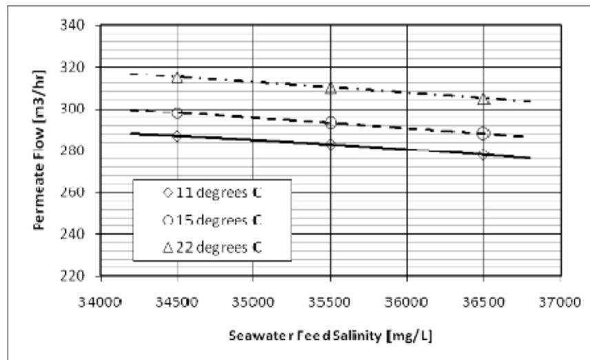
Figure 10 – Modeled Permeate Flow versus Salinity and Temperature
