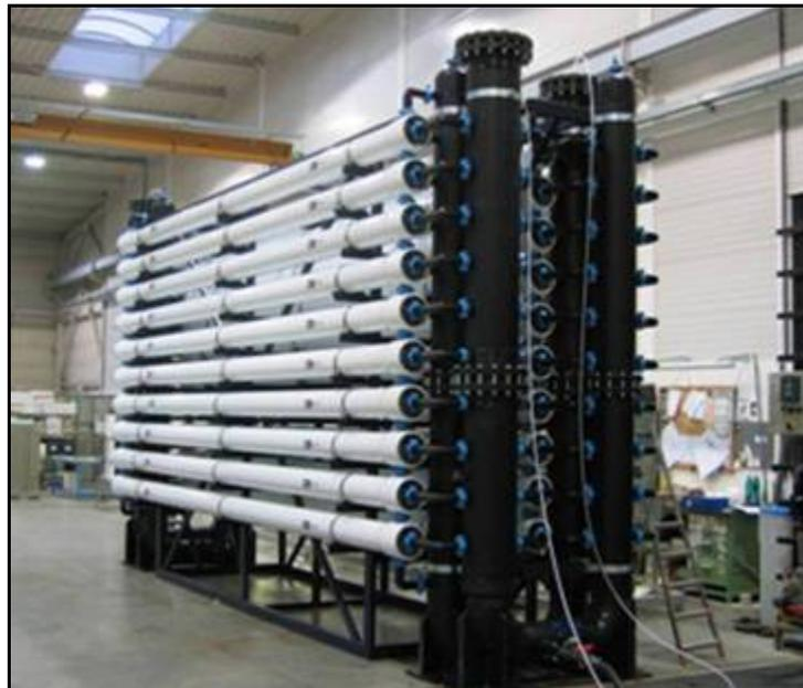
Figure 4 – NORIT Seaguard Ultrafiltration Skid
