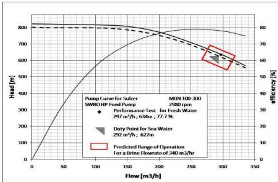
Figure 11 – Range of Operation of the High Pressure Feed Pump
