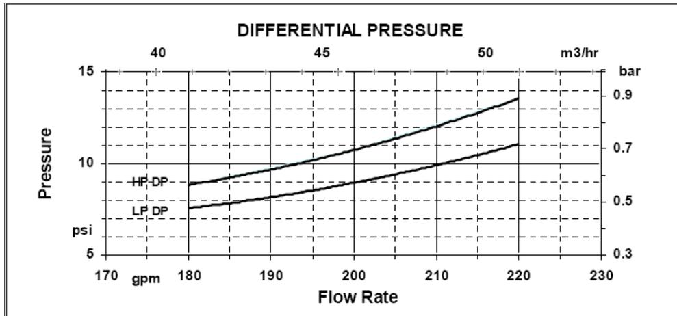
Figure 8 – Typical PX220 Device Characteristic curves
