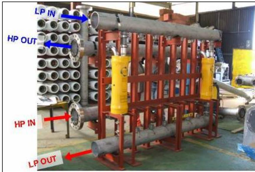
Figure 9 – ERD array with frame for 8 PX units in parallel (during construction)
