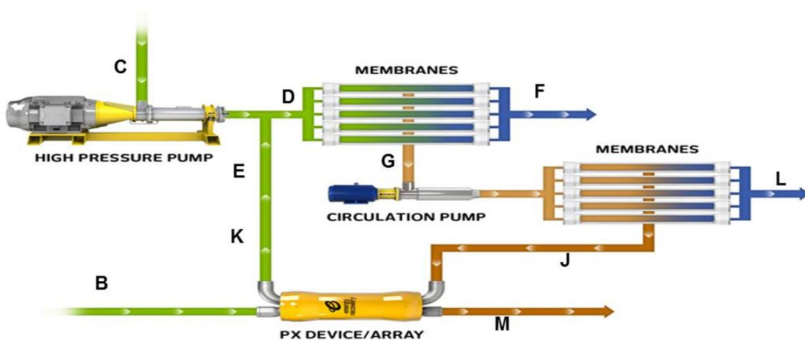
**Figure 1.** Typical PX device Installation for 2-stage BWRO
