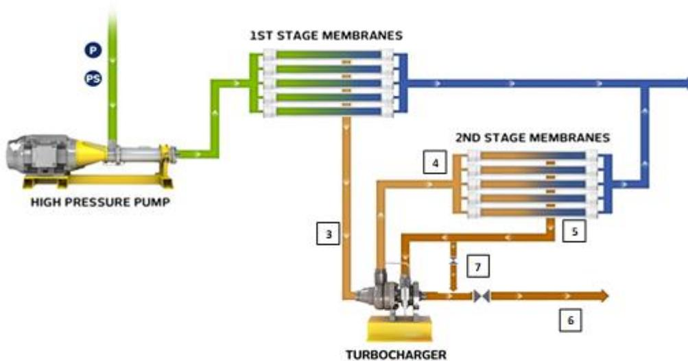
**Figure 3.** Typical turbocharger Installation for 2-stage BWRO
