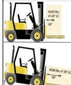
Improperly distributed loads may tip the forklift because the center of gravity has shifted
