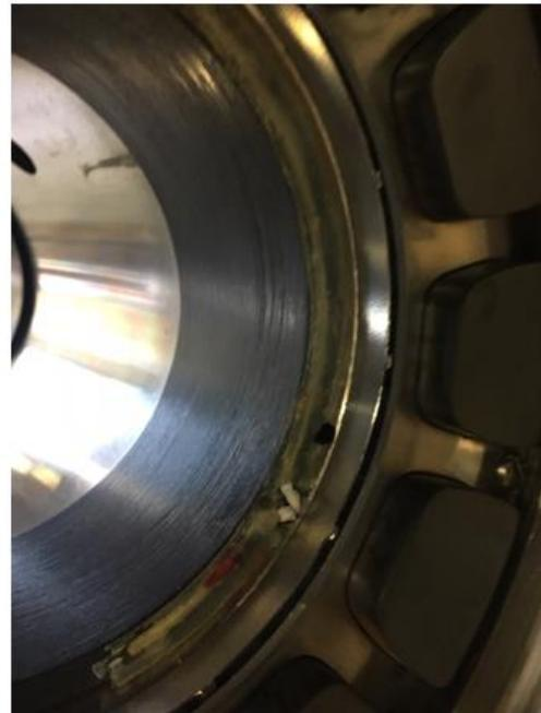
b) Journal bearing in good condition after lab mechanical run test
