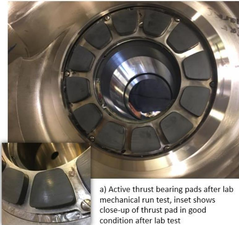
a) Active thrust bearing pads after lab mechanical run test, inset shows close-up of thrust pad in good condition after lab test
