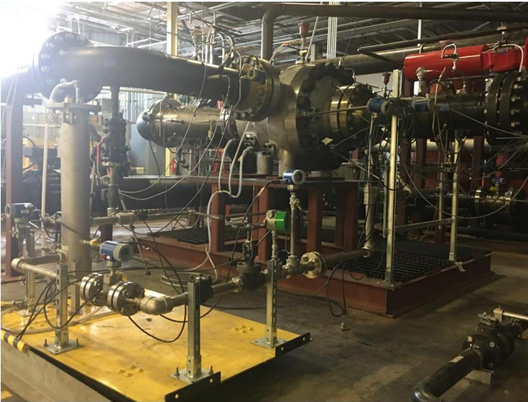
Figure 32: Turbocharger FAT setup with lubrication skid in the foreground
