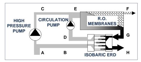
Figure 3: Simplified Diagram of an RO Process with Isobaric ERDs
