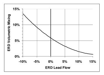
Figure 4 – ERD Mixing Versus Lead Flow
