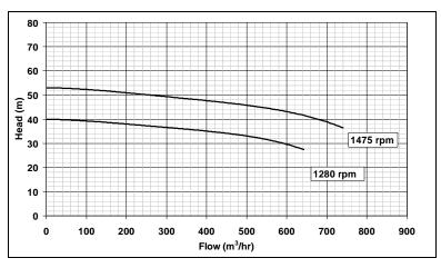
**Figure 6 – Circulation Pump Characteristic Curves**
