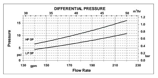
Figure 7 – PX-220 ERD Characteristic Curves
