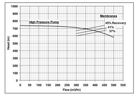
**Figure 5 – High-Pressure Pump and Membrane Characteristic Curves**
