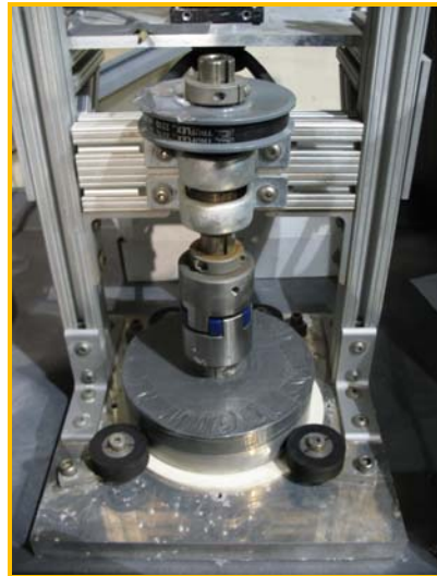
FIGURE 2. ERI Submersible “Pin on disk” Ceramic wear testing apparatus
