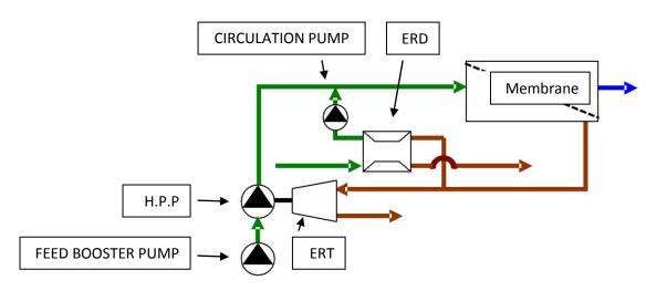
Figure 4 – 4A SWRO Train after Hybrid Retrofit,
