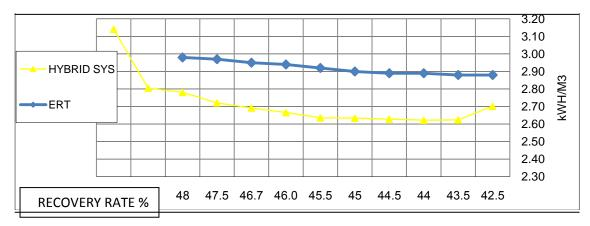
Figure 5 –SWRO Specific Energy Consumption ERT VS Hybrid system as measured in Palmachim.
