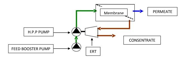
Figure 1 – SWRO Train with Original ERT Design
