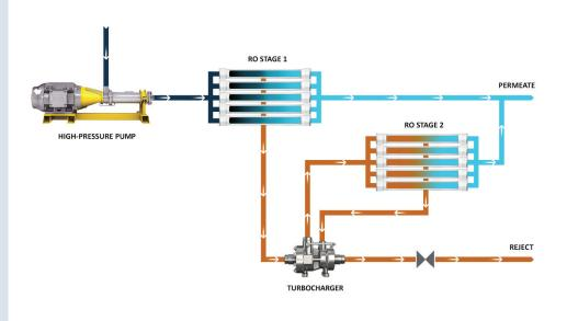
Energy Recovery's turbochargers save energy and help balance the flux between stages, extending the life of the membrane system and ultimately resulting in increased uptime. The rate of fouling and replacement also decreases, leading to fewer maintenance issues and increased operational savings.
